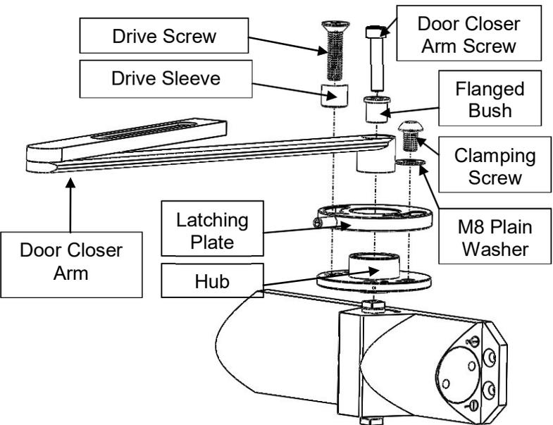
\* The maximum latch angle is limited by the depth of the architrave around the door, and by any obstruction behind it
