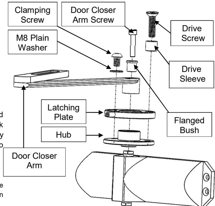
\* The maximum latch angle is limited by the depth of the architrave around the door, and by any obstruction behind it
