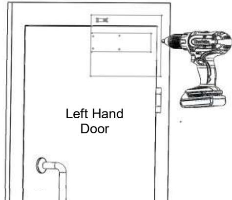
Fit the closer baseplate securely to the door using the 4 x N°8 \* 1-1/4" screws. Place the free end of the spring over the topmost pillar on the baseplate
