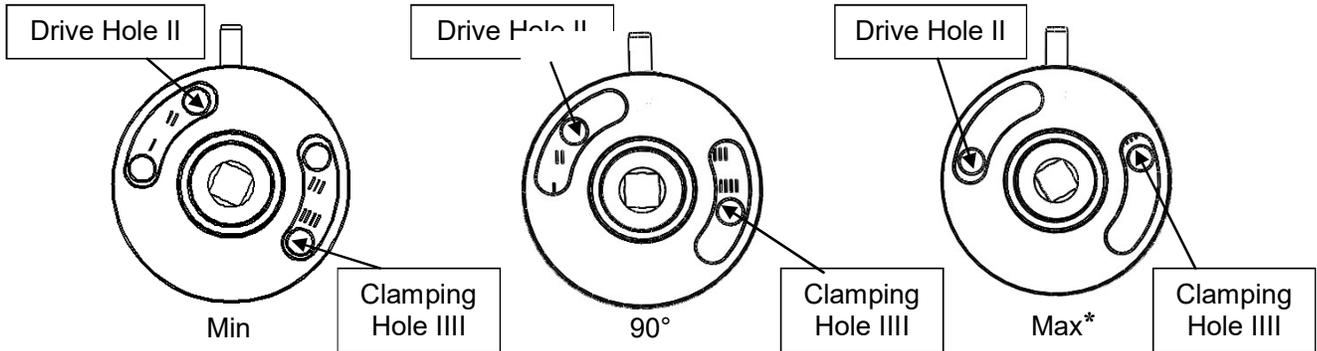
*Figure 2: Right Hand Projecting Arm Cam Positions*
